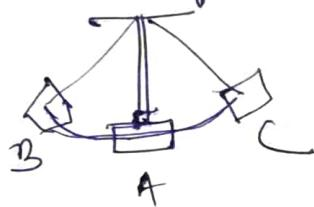
Torsional vibration - if the shaft gets alternatively twisted and untwisted on account of an alternate torque on the disc, is said to execute torsional vibration.
