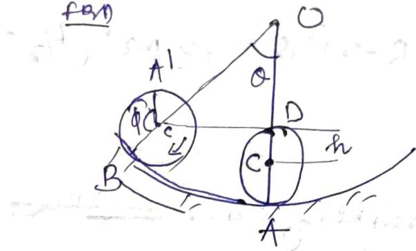
when the cylinder rolls on a circular surface and takes the new position.
