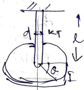
Suppose a system, having a body of mass moment of inertia  $I$  connected to shaft (at its end) of torsional stiffness  $k_T$ , is twisted by an angle  $\theta$ .
