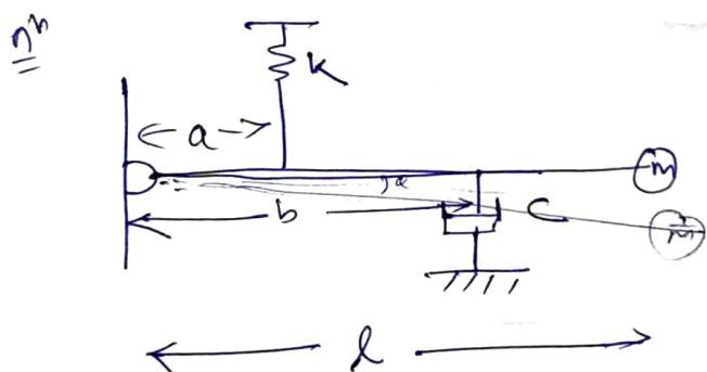
Equation of motion, when small angular displacement is given.
