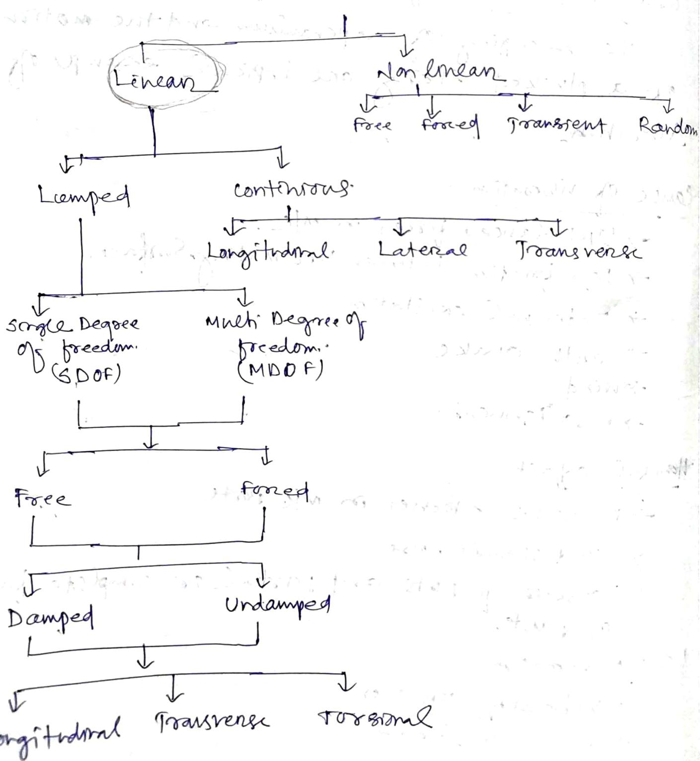
Linear vibration :- If all the basic element of vibrating system ie mass, spring and damper behaves linearly called linear vibration. The differential equation of the system are linear.
