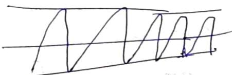
Random vibration - if the magnitude of excitation acting on the vibratory system at a given time cannot be predicted, the resulting vibration is known as random vibration or non-deterministic vibration.
