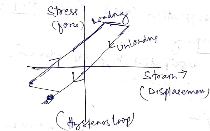
The area of this loop is the amount of energy dissipated in one cycle during vibration. This type of loop is known as hysteresis loop.
