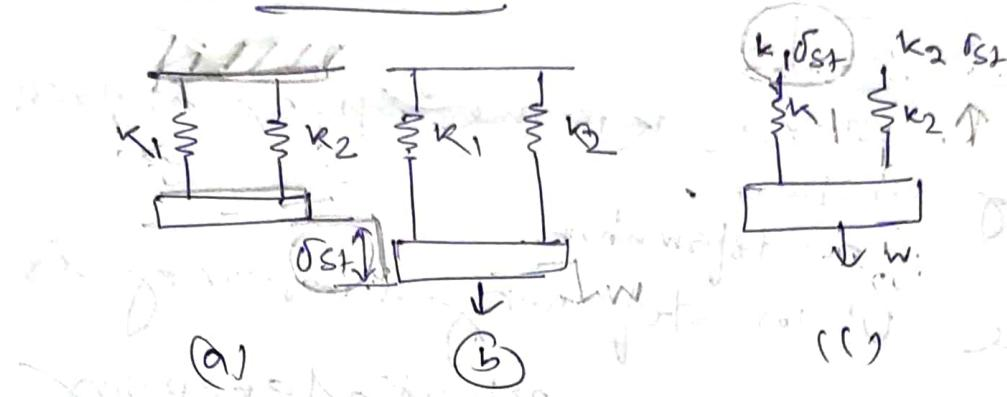
when the load applied, the system undergoes a static deflection  $\delta_{st}$ . For FBD
